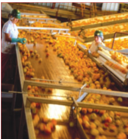
Sorting for just the right size: high-speed conveyor belt & canning plant staff select the best peaches for canning.
